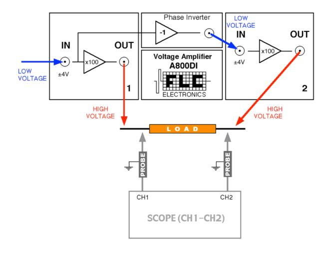
REMEMBER: There cannot be any connection between the load and ground!
