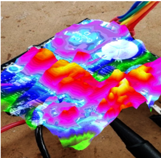
FIGURE 1. An overlapped 3D radiation pattern as obtained from the Detectus sw application.
