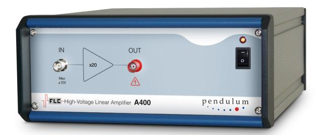
The Pendulum Instruments High Voltage Linear Amplifier A400 has a fixed amplification of 20 times and capable of bipolar high voltage output of  $\pm 200$ . Any other signal source with amplitude up to  $\pm 10$  V can be used as an input device. The input amplitude should normally be kept within  $\pm 7.5$  V. The A400 High Voltage Linear Amplifier is equipped with a microfuse rated at 15 mA, which will be blown if the input voltage exceeds 300% of the maximum.
