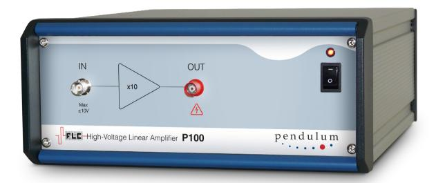
The Pendulum Instruments High Voltage High Current Linear Amplifier P100 has a fixed amplification of 10 times and capable of bipolar high voltage output of  $\pm 50$ V. Any signal source with amplitude up to  $\pm 10$  V can be used as an input device. The input amplitude should normally be kept within  $\pm 10$  V. The High Voltage High Current Linear Amplifier P100 is equipped with a microfuse rated at 15 mA, which will be blown if the input voltage exceeds 300% of the maximum.
